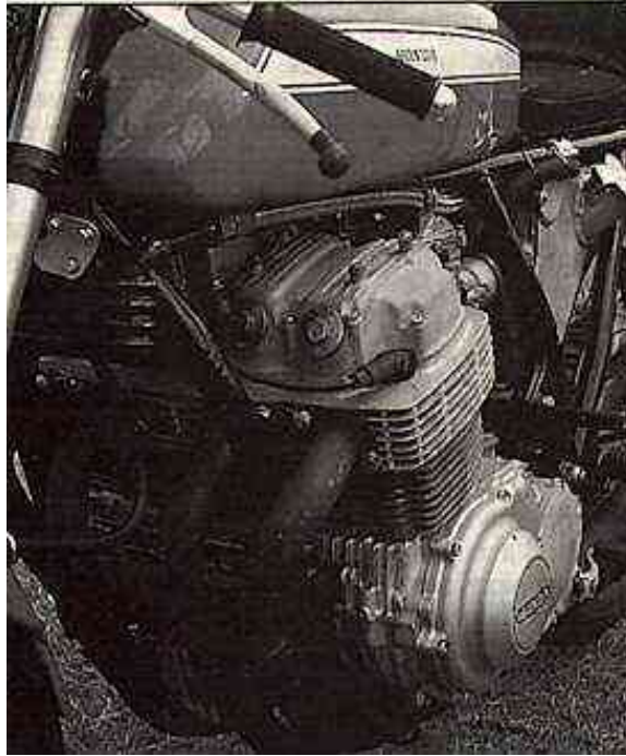
A close-up of Dick Mann's 1971 Daytona-winning Honda CR 750, showing the slimmed-down race-only alternator.
